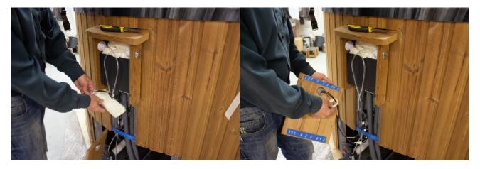
Remove the wires from the insulation, unscrew the nut retaining the control panel for the LED light and disconnect the wires.
